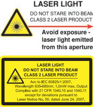
Figure 2. FDA (CDRH) warning label (Class 2)
